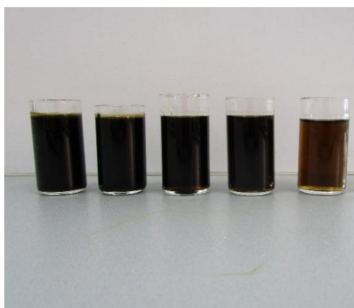
Fig. S1: Five specimens with different concentrations of GO and OapPOSS, denoted by GOPOS90, GOPOS70, GOPOS50, GOPOS30, and GOPOS10 sol (from left to right).
