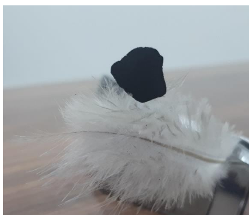
Fig. S3: Ultralight-weight obtained aerogel located on a very light feather.
