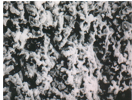
Fig. 8: SEM micrograph of Secar71 hydrated for 90 days at 36 °C ----- 30um
