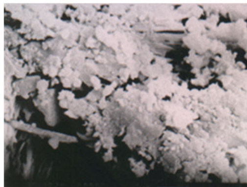
Fig. 2: SEM micrograph of Secar71 hydrated for 9 days at 28 °C ----- 3um.
