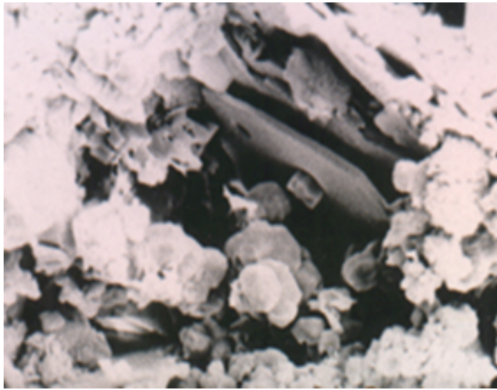
Fig. 7: SEM micrograph of Secar71 hydrated for 7 days at 36 °C ----- 3um.
