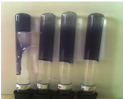
Fig. 7: Effect of water formation as an in situ reservoir fluid on gel polymer properties after 15 hours aging at ambient temperature.
