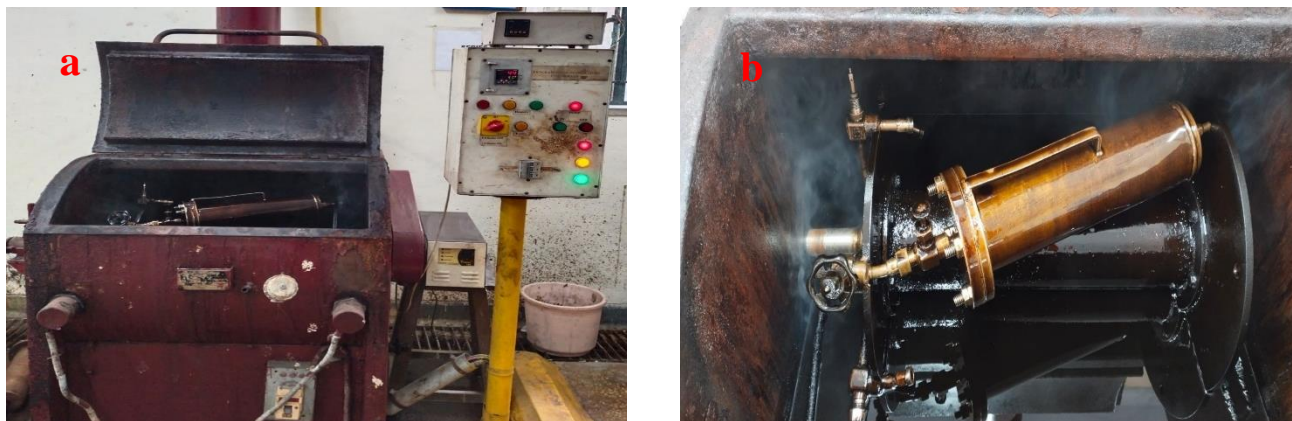
Fig. 1: (a) Series Digester used for LHT of bagasse BL (b) Bomb inside digester filled with SCBL
