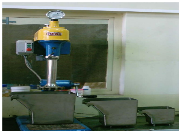
Fig. 1: Scheme of Denver flotation device.
