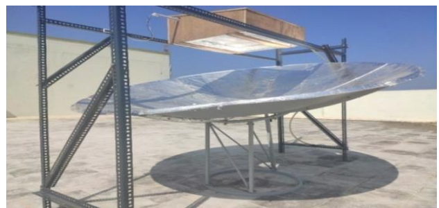
Fig. 5: Condition 4 – Solar Still With Insulation-With Dish (WI-WD)
