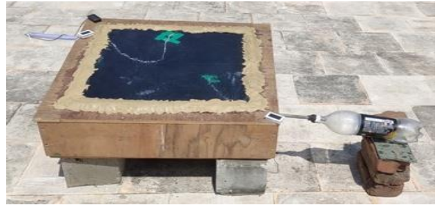
Fig. 2: Solar still with insulation and without Dish (WI-WoD)
