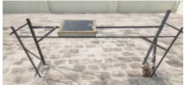
Fig. 3: Solar still without insulation and without dish (WoI-WoD)
