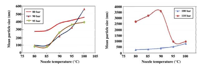
Fig. 2: Mean particle size changes with nozzle temperature.
