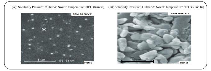
Fig. 3: SEM images of the particle, formed in (A); run 6 and (B); run 16.
