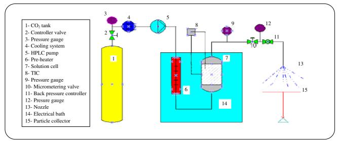
Fig. 1: RESS Apparatus.
