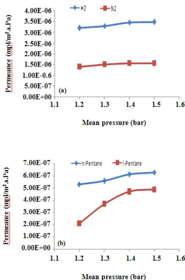
Fig. 5: Single gas permeance a) H<sub>2</sub> and N<sub>2</sub> and b) pentane isomers through MFI zeolite membrane (with four hydrothermal synthesis steps, calcined at 673K for 30h) as a function of mean pressure at 100 °C.
