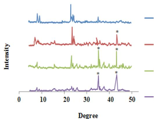
Fig. 1: XRD patterns of the silicalite-1 / $\alpha$ -alumina composite membranes at the first (a); second (b); third (c) and fourth (d) hydrothermally synthesized layers (the peaks originating from the  $\alpha$ -alumina support were labeled with '\*').
