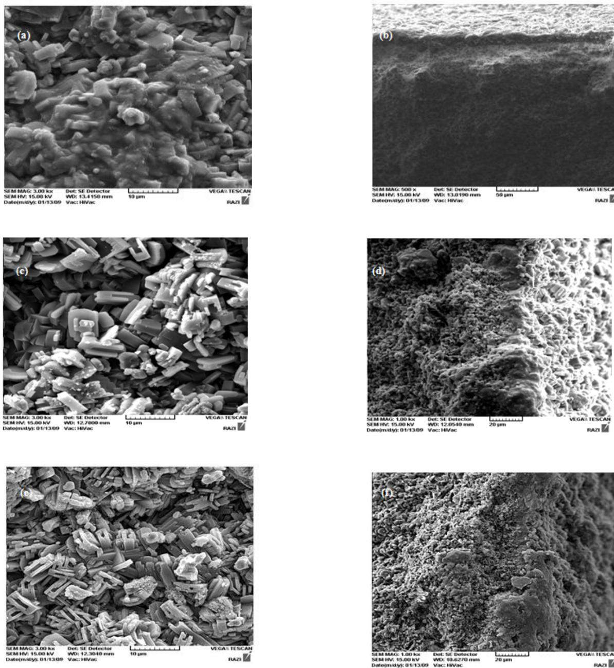
**Fig. 4:** SEM micrographs of the supported MFI zeolite membrane (with four hydrothermal synthesis steps): surface and cross section of the membranes calcined at 673K after different calcination times 4 h (a,c); 8h (c,d); 30 h (e,f).
