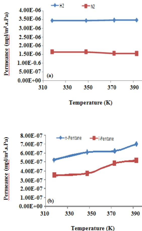
Fig. 6: Single gas permeance a) H<sub>2</sub> and N<sub>2</sub> and b) pentane isomers through MFI zeolite membrane (with four hydrothermal synthesis steps, calcined at 673K for 30h) as a function of temperature at 1 bar.
