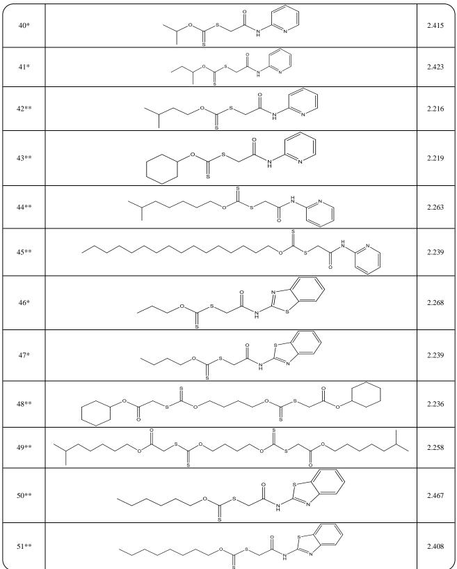
Table 1: Experimental lubricant additives onset temperature ( $T_{onset}$ ), (Continued).
