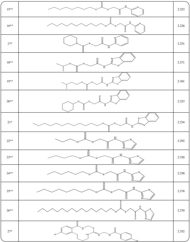
Table 1: Experimental lubricant additives onset temperature ( $T_{onset}$ ), (Countinued).
