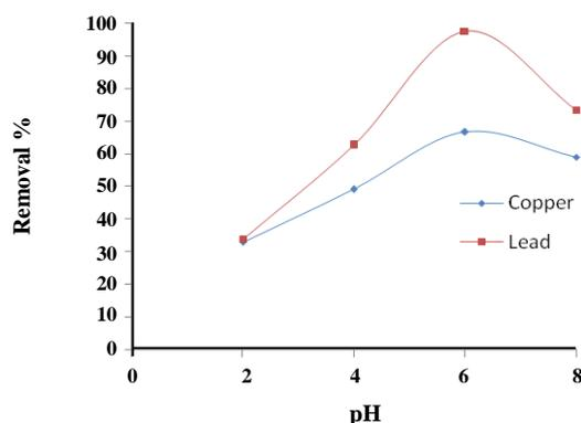
Fig. 1: Effect of pH on the adsorption of lead (II) and copper (II) (Conditions: 0.8g adsorbent dosage, 160 rpm, 2 hours agitation time, temperature 25 °C) [one experimental run for each graph, an average of three AAS measurements for each data point].
