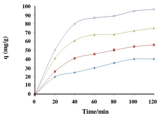
Fig. 3: Effect of contact time at the differential initial concentration on the adsorption of lead (II) (Conditions: 0.8g adsorbent dosage, 160 rpm, 2 hours agitation time, temperature 25 °C) [one experimental run for each graph, average of three AAS measurements for each data point].
