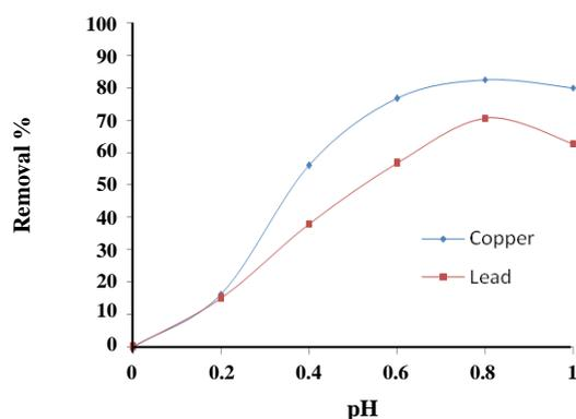
Fig. 2: Effect of adsorbent dosage on the adsorption of lead (II) and copper (II) (Conditions: 25ppm lead & 2 ppm copper, 160 rpm, 2 hours agitation time, temperature 25 °C) [one experimental run for each graph, average of three AAS measurements for each data point].
