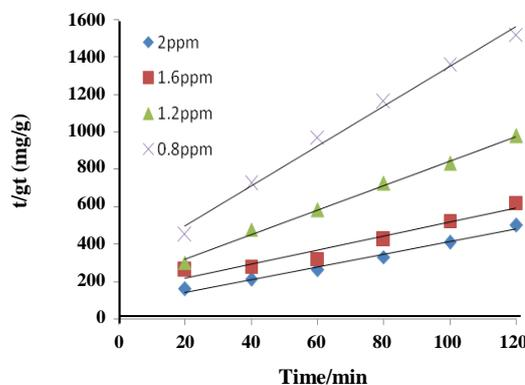
**Fig. 8: Pseudo second-order plot for the adsorption of copper (II) on sodium bentonite/carbon black composite adsorbent (Conditions: 0.8g adsorbent dosage, 160 rpm, and temperature 25 °C).**
