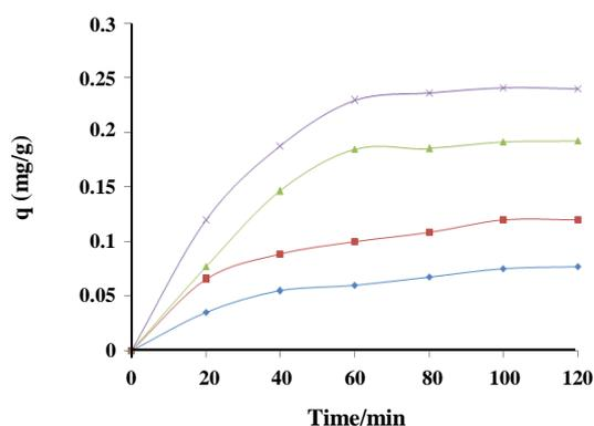
Fig. 4: Effect of contact time at the differential initial concentration on the adsorption of copper (II) (Conditions: 0.8g adsorbent dosage, 160 rpm, 2 hours agitation time, temperature 25 °C) [one experimental run for each graph, average of three AAS measurements for each data point].
