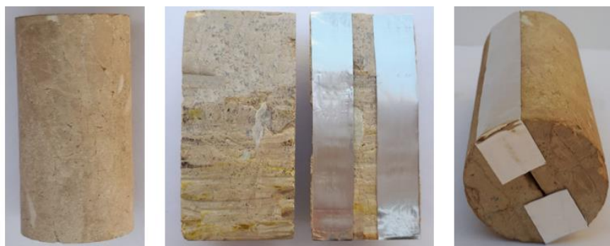
Fig. 1: Schematic of the fractured core model used in the coreflooding test.
