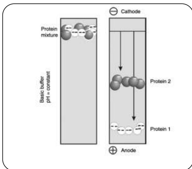
**Fig. 2: Separation principle of the electrophoresis process. Proteins with different net charges and sizes migrate in an electric field in the presence of a buffer with different migration velocities. Different proteins form discrete zones [47].**
