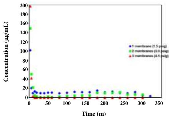
Fig. 8: Optimized ultrafiltration for separating BSA and bovine serum albumin at different pressures: by utilizing three stacked membranes the total rejection of serum albumin is obtained [44].
