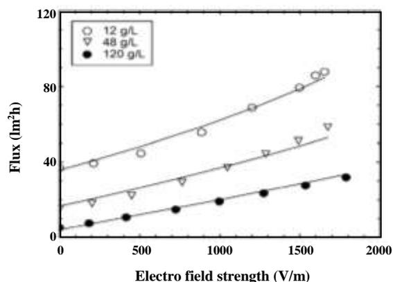
Fig. 11: Flux enhancement by applying an electric field for three different concentrations of solution. The solid lines represent experimental model ( $TMP=1.5$  bar,  $v=0.07$  m/s) [123].
