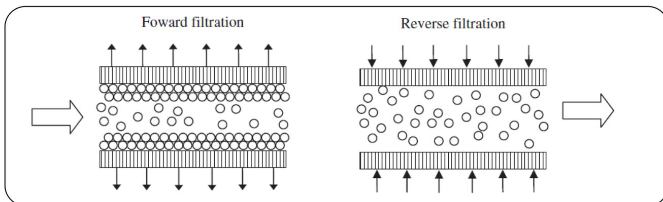
Fig. 5: Schematic representation of forward and reverse filtrations [123].
