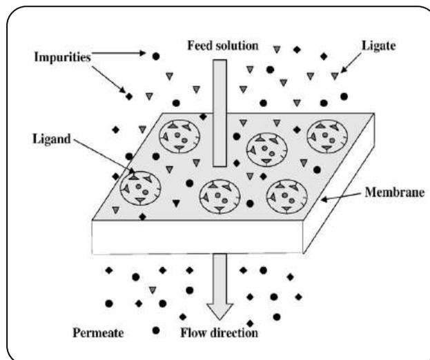
Fig. 4: Schematic representation of membrane chromatography process [22].
