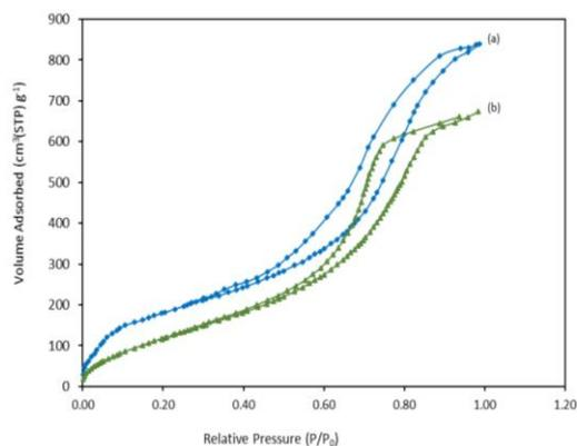
**Fig. 4: N<sub>2</sub> adsorption- desorption isotherms of (a) pure silica aerogel (b) magnetic silica aerogel.**
