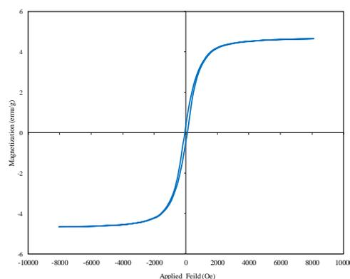
**Fig. 6:** Room temperature (298K) magnetization curve for magnetic silica aerogel nanocomposite.
