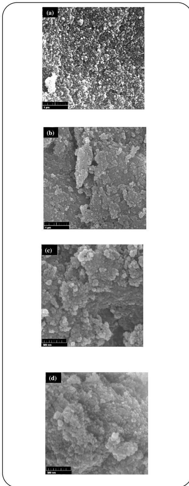
**Fig. 3: FESEM micrographs of (a) silica aerogel; (b) silica aerogel-pectinase; (c) magnetic silica aerogel and (d) magnetic silica aerogel-pectinase**
