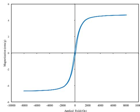
**Fig. 6:** Room temperature (298K) magnetization curve for magnetic silica aerogel nanocomposite.
