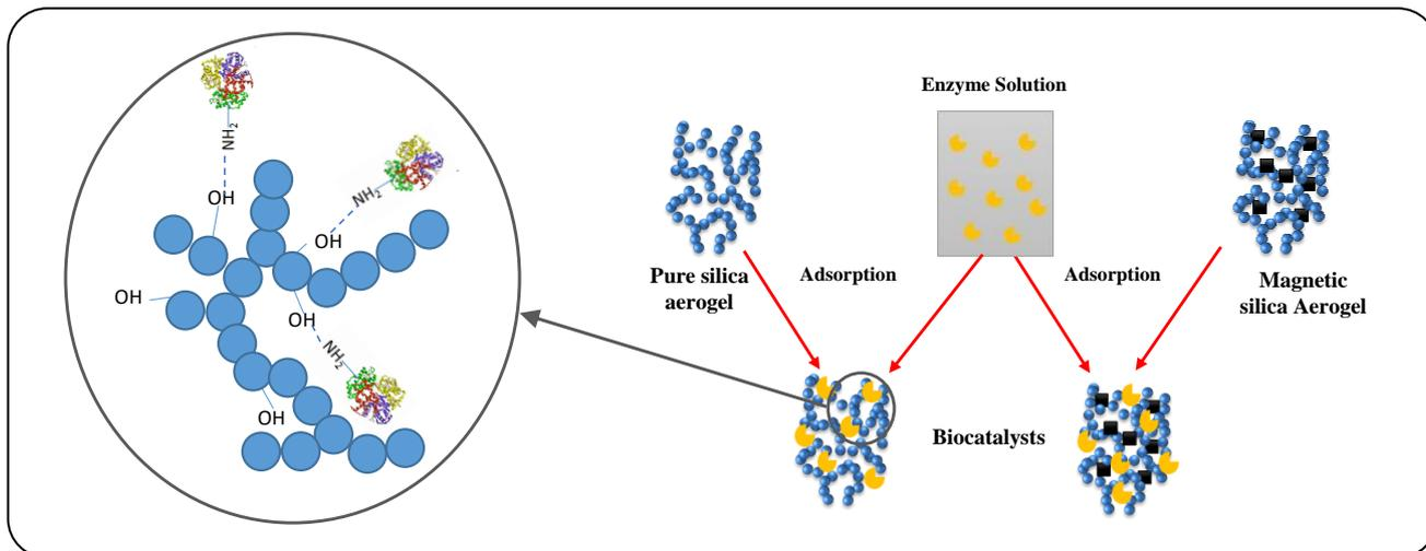
Fig. 2: Schematic representation of the synthesis of biocatalysts
