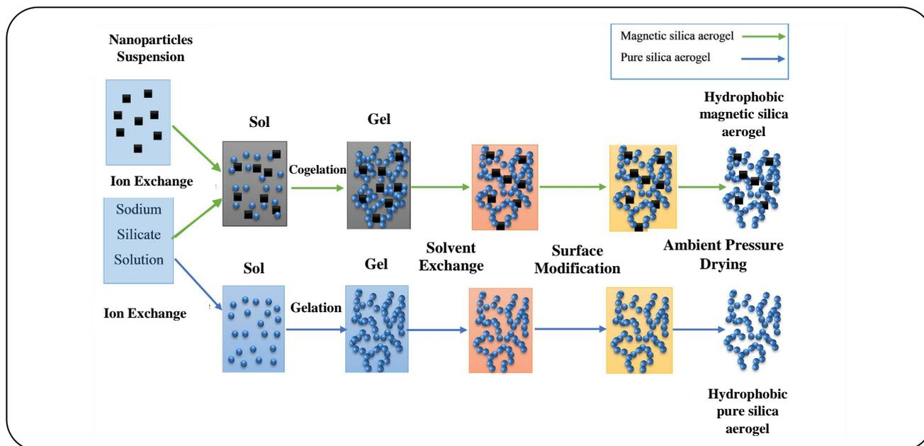
Fig. 1: Schematic representation of the synthetic procedure of pure and magnetic silica aerogels.
