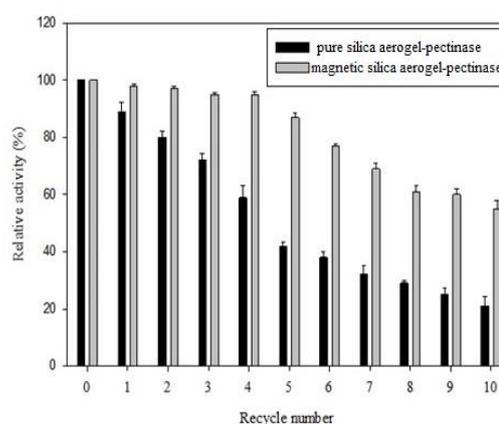
**Fig. 11. Reusability of immobilized pectinase on pure silica aerogel ■ Magnetic silica aerogel■.**
