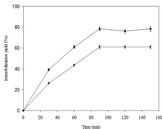
**Fig. 7:** The effect of immobilization time on the pectinase adsorption onto pure silica aerogel ■ Magnetic silica aerogel ●.
