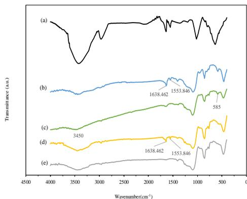
**Fig. 5: FT-IR spectra of the supports before and after immobilization: (a) free pectinase (b) magnetic silica aerogel-pectinase, (c) magnetic silica aerogel (d) silica aerogel-pectinase (e) pure silica aerogel.**
