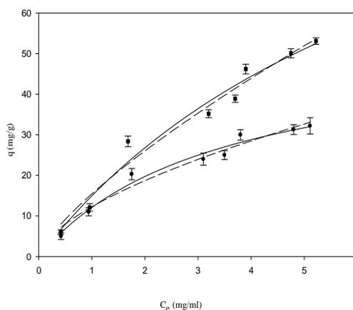
**Fig. 9. Adsorption equilibrium of pectinase on pure silica aerogel ■ Magnetic silica aerogel ● at ambient temperature (solid line for Langmuir model, dashed line for Freundlich model).**
