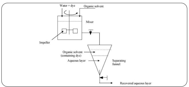
Fig. 1: Schematic experimental setup for liquid-liquid extraction for removal of dye from aqueous solution.
