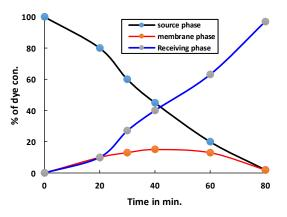
Fig. 8: Effect of time (volume of source phase 260 mL of 50 mg/L of dye at pH 7± 0,1 carrier concentration  $4.48 \times 10^{-1}$  mol/L, volume of receiving phase 260 mL of 1N H<sub>2</sub>SO4 and rate of stirring 400rpm).
