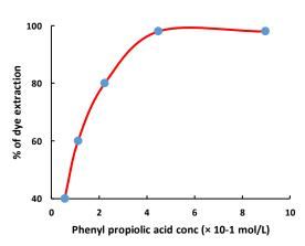
Fig. 4: Effect of carrier concentration (feed 25 mL of 50 mg/L of dye at pH 7  $\pm$  0.1, the volume of organic phase 25 mL, equilibration time 3 min).
