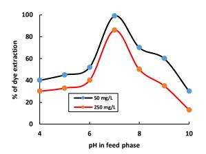
Fig. 5: Effect of pH of feed phase (volume of source phase 260 mL of 50 mg/L and 250 mg/L of dye at various, pH carrier concentration  $4.48 \times 10^{-1}$  mol/L, volume of receiving phase 260 mL of 1 N H<sub>2</sub>SO<sub>4</sub>, rate of stirring 400 rpm and effect of time 70 min.
