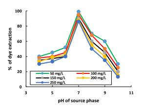
Fig. 3: Effect of pH in source phase( volume of feed 25 mL, carrier concentration  $4.48 \times 10^{-1}$  mol/L, volume of organic phase 25 ml and equilibration time 3 min).
