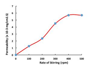
Fig. 5: Effect of stirring speed (volume of source phase 260 mL of 50 mg/L of dye at pH 7 ± 0.1, carrier concentration  $4.48 \times 10^{-1} \text{ mol/L}$ , volume of receiving phase 260 mL of 1N H<sub>2</sub>SO<sub>4</sub>, and effect of time 70 min).
