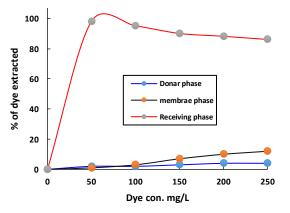
Fig. 7: Effect of dye concentration (volume of source phase 260 mL of different concentration of dye at pH 7± 0,1 carrier concentration 4.48 × 10<sup>-1</sup> mol/L, volume of receiving phase 260 mL of 1N H<sub>2</sub>SO<sub>4</sub>, rate of stirring 400rpm and effect of time 70 min).
