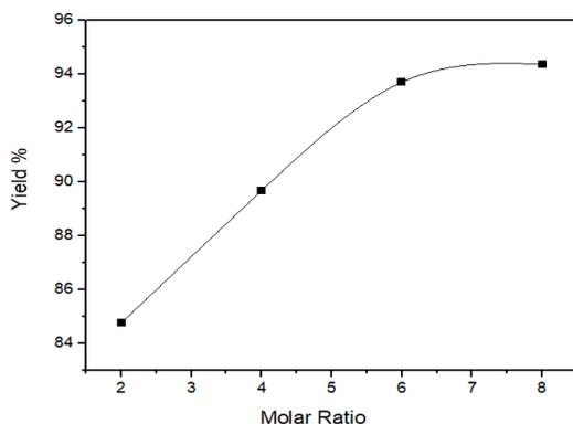
**Fig. 5:** Effect of molar ratio (ethylene glycol) on production yield of Bio lube.
