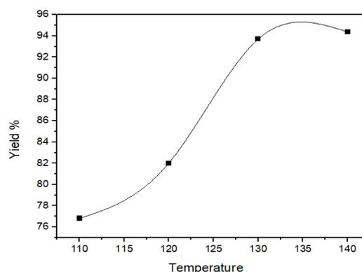
**Fig. 4: Effect of Reaction Temperature on production yield of bio lube.**
