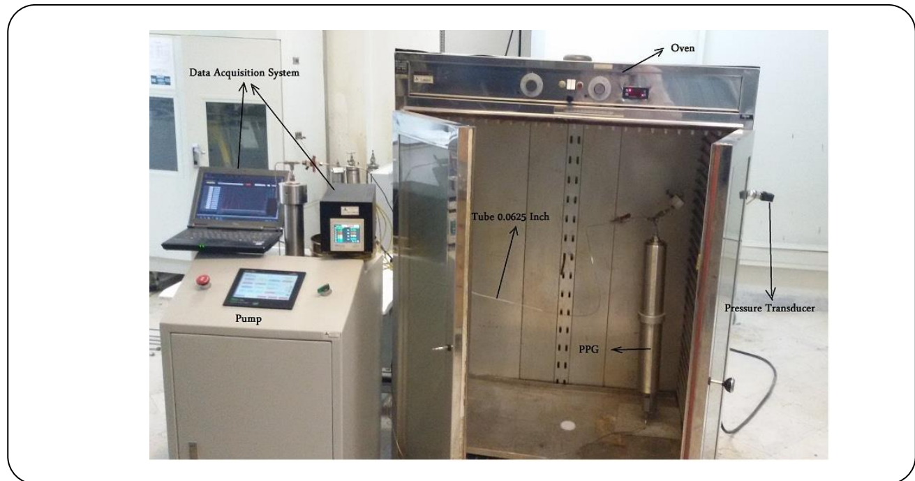
Fig. 2: The schematic diagram of the experimental set up- Viscosity Test.
