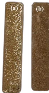
Fig. 4. a) R-EPS containing 3 wt. % treated STLP b) R-EPS containing 5 wt. % treated STLP
