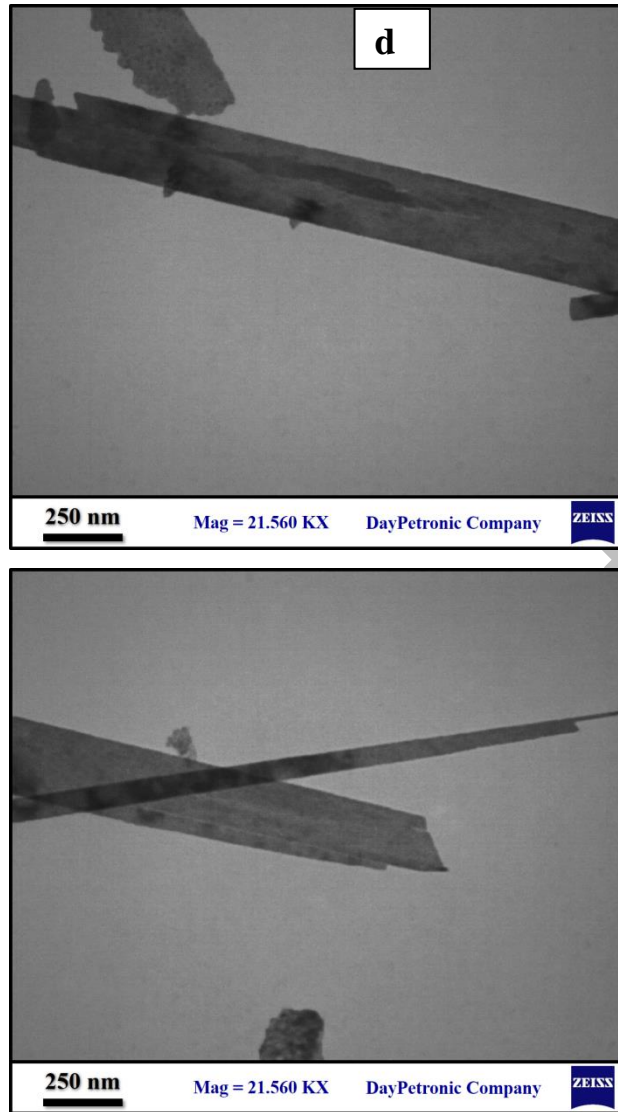
Fig. 2 SEM (a, b) and TEM (c, d) images of \text{CeO}_2/\text{Bi}_2\text{WO}_6 nanocomposite.
