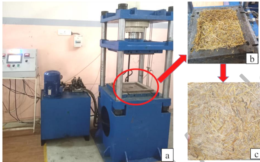
Fig. 6: Image of the composite fabrication (a) Compression molding machine (b) Mould (c) Laminate
