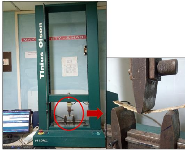
Fig. 9: Photographic image of the flexural test machine
