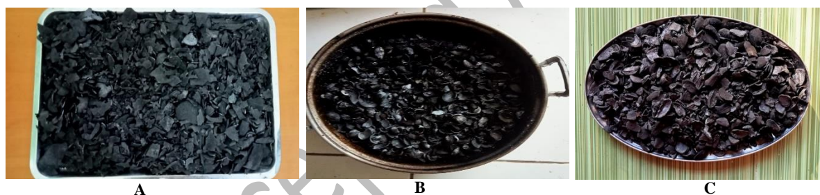
Fig. 3: The results of carbonization operations using coconut shells (A), nutmeg shells (B), and canary shells (C).
