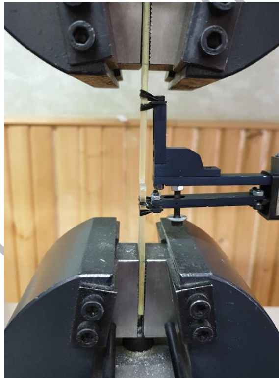
Figure 3: Tensile testing setup showing a specimen mounted in the tensile testing grips.
