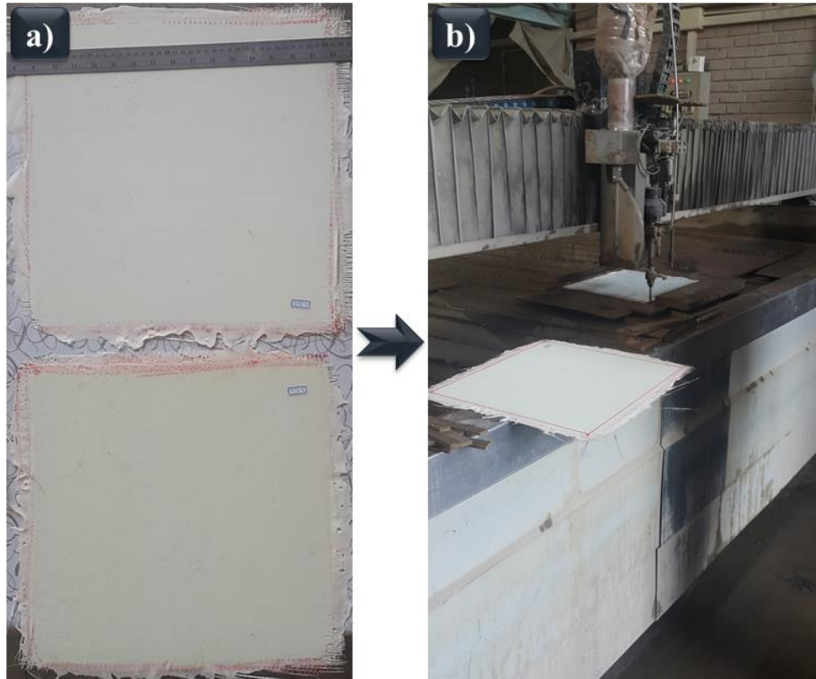
Figure 2: a) Composite coating specimens reinforced with HA nanofibers, labeled based on fiber content and substrate type, and b) cutting specimens based on test's standards for evaluating mechanical properties.
