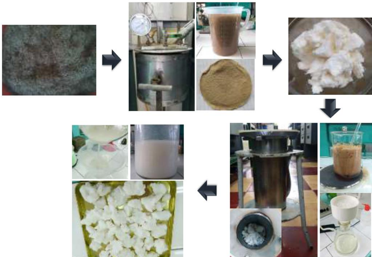
Fig. 4: Production process for sugarcane bagasse nanocellulose [165]
