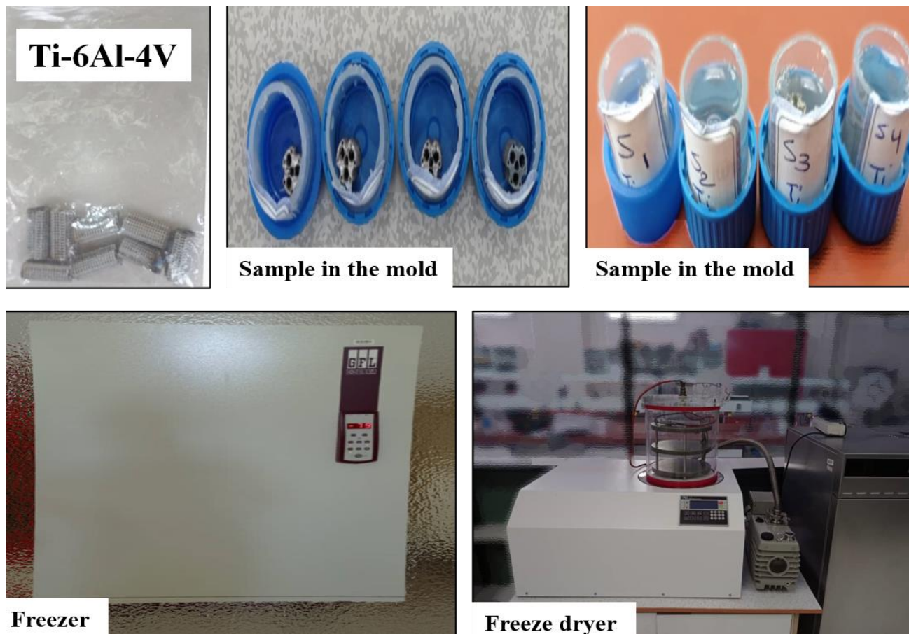
Fig. 1: The manufacturing process of metal scaffold with chitosan-wollastonite polymer coating for use in the treatment of bone fractures.
