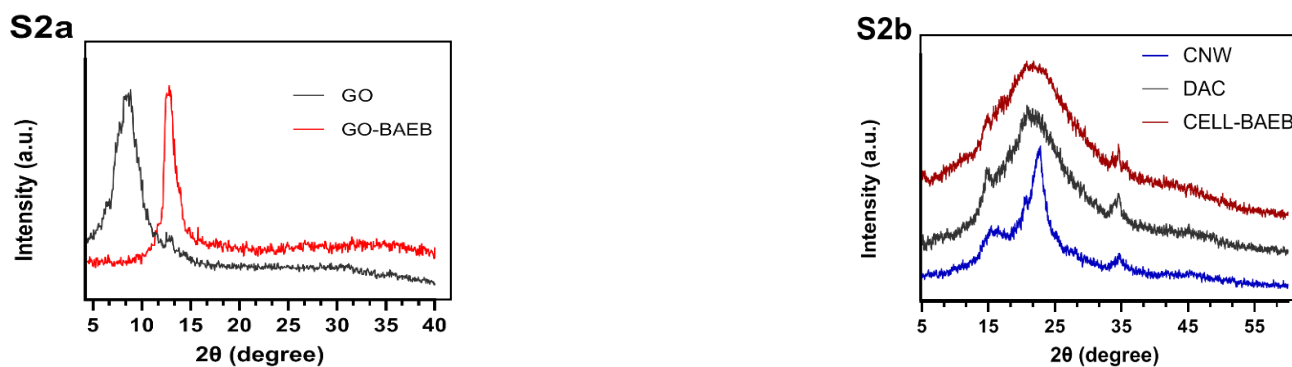
Fig. S2a) XRD patterns of GO, GO-BAEB and S2b) CNWs, DAC, and CELL-BAEB
