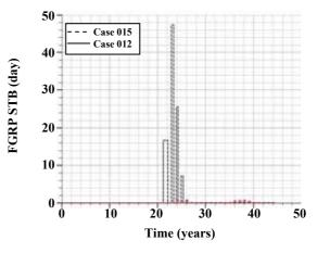
Fig. 5: Comparison of water production for models 012 and 015.
