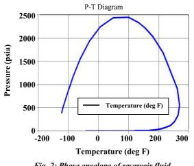
Fig. 2: Phase envelope of reservoir fluid
