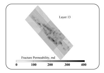
Fig. 6: Distribution of fracture permeability in different layer 13.
