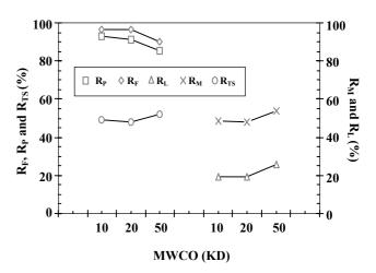
Fig. 8: The effect of MWCO on solutes rejection (protein,  $R_P$ ; Fat,  $R_F$ ; Lactose,  $R_L$ ; Mineral,  $R_M$  and Total Solids,  $R_{TS}$ ) during ultrafiltration of skim milk.
