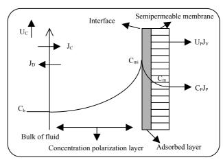
Fig. 1: Schematic presentation of hydraulic resistances based on adsorption-boundary layer model.
