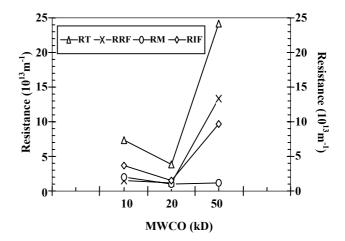
Fig. 6: The effect of MWCO on total hydraulic resistance  $(R_T)$ , reversible fouling resistance  $(R_{rf})$ , irreversible fouling resistance  $(R_{if})$  and membrane hydraulic resistance  $(R_m)$  during ultrafiltration of skim milk.
