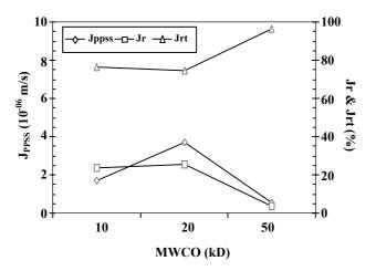
Fig. 4: The effect of MWCO on pseudo steady state flux  $(J_{ppss})$ , relative flux  $(J_r)$  and total relative flux decline  $(J_{rl})$  during ultrafiltration of skim milk.
