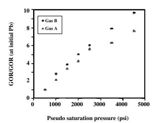
Fig. 1: GOR changes due to gas dissolution in Oil A.
