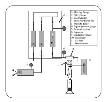
Fig. 10: Schematic representation of set up used in gas injection.
