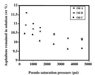
Fig. 14: Remained asphaltene in solution during injecting different volume of Gas A.
