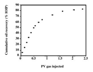
Fig. 11: Oil recovery during gas injection in the physical model.
