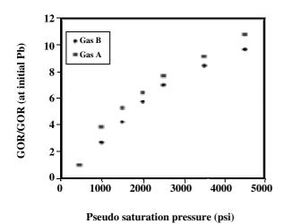
Fig. 2: GOR changes due to gas dissolution in Oil B.
