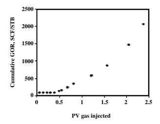
Fig. 12: Gas /oil ratio during gas injection in the physical model.
