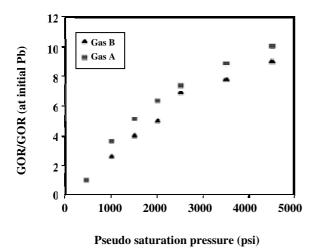
Fig. 3: GOR changes due to gas dissolution in Oil C.
