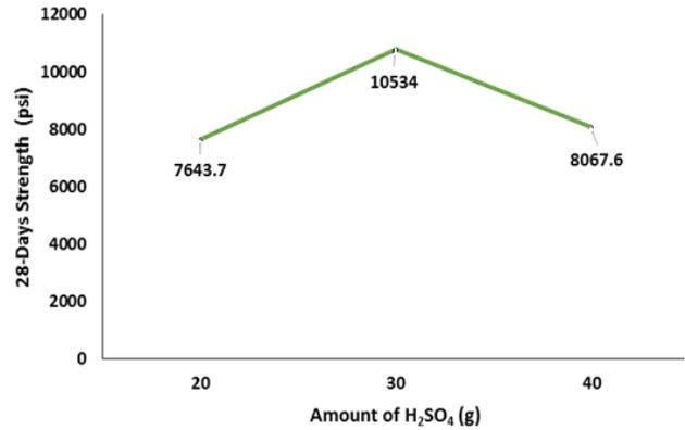
Fig. 7: Strength at various dosages of  $H_2SO_4$
