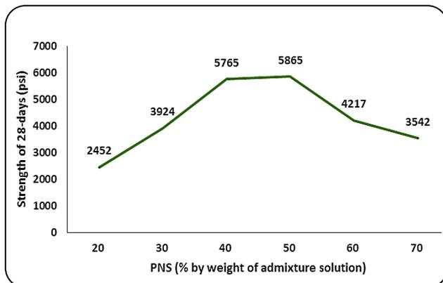
**Fig. 4: Amount of PNS in solution and strength**
