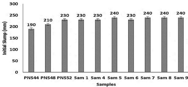
Fig. 5: Comparison of all samples for the initial slump
