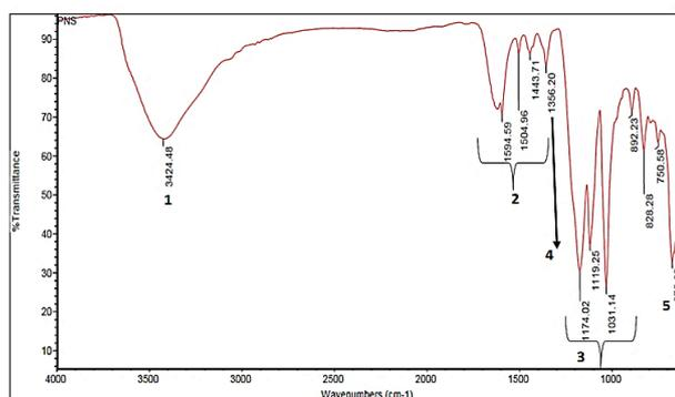
Fig. 3: FTIR Poly-naphthalene sulphonate
