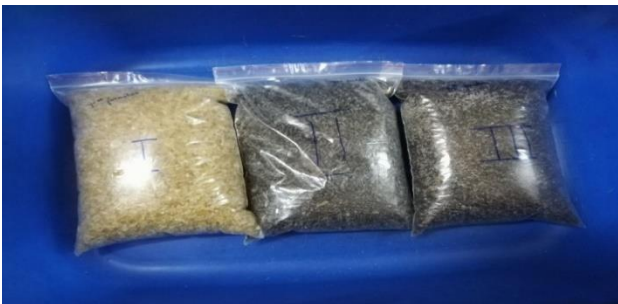
Fig. 6: Extruded composite from twin extruder
