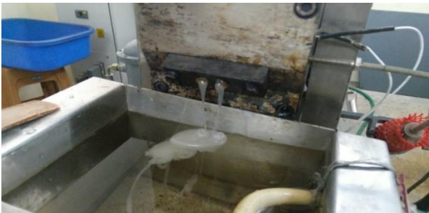
Fig. 6: Extruded composite from twin extruder
