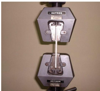
Fig. 14: Loading arrangements for tensile test
