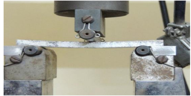
Fig. 17: Loading arrangements for flexural test
