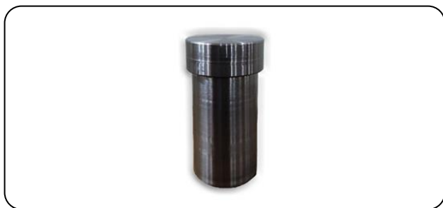
Fig. 1: Cylinder made of stainless steel 316L.
