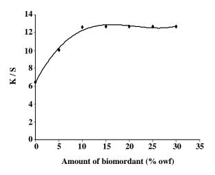
Fig. 1: Effect of the amount of biomordant on the color strength of dyed wool at pH= 5.
