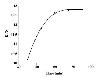
Fig. 4: Effect of dyeing time on color strength of dyed wool.
