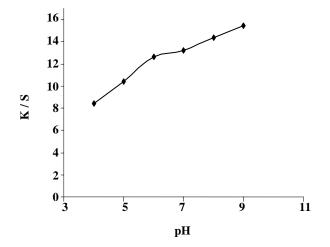
Fig. 2: Effect of pH on color strength of dyed wool.
