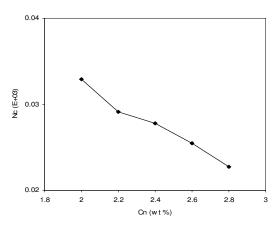
Fig. 13: Capillary number in viscous-modified surfactant waterflooding versus NaCl concentration (MgCl<sub>2</sub>: 0.5 wt.%, CaCl<sub>2</sub>: 0.5 wt.%). Concentrations of chemicals in polymersurfactant solution in surfactant waterfloods are: surfactant = 0.10 wt.%, Xanthan = 125 ppm, and ethanol = 0.75 wt.%.
