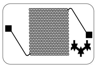
Fig. 2: A schematic of one-quarter five-spot glass micromodel with a magnified view of its pores.
