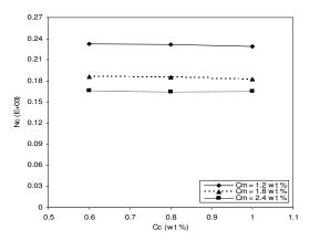
Fig. 7: Capillary number in viscous-modified surfactant waterflooding versus  $CaCl_2$  concentration (first range) for three concentrations of  $MgCl_2$ . Concentrations of chemicals in polymer-surfactant solution in surfactant waterfloods are: surfactant = 0.10 wt.%, xanthan = 125 ppm, and ethanol = 0.75 wt.%.
