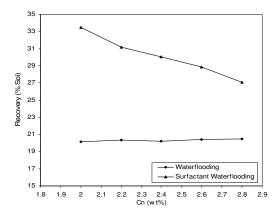
Fig. 10: Ultimate oil recovery in waterflooding and viscous-modified surfactant waterflooding versus NaCl concentration ( $MgCl_2 = 0.5$  wt.%,  $CaCl_2 = 0.5$  wt.%). Concentrations of chemicals in polymer-surfactant solution in surfactant waterfloods are: surfactant = 0.10 wt.%, xanthan = 125 ppm, and ethanol = 0.75 wt.%.
