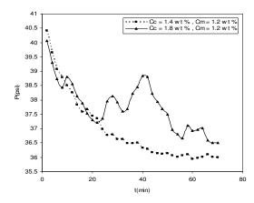
Fig. 9: A typical injection pressure response versus time in the third range of CaCl<sub>2</sub> concentration during the viscous-modified surfactant waterflooding of a porous network filled with connate water and heavy oil.
