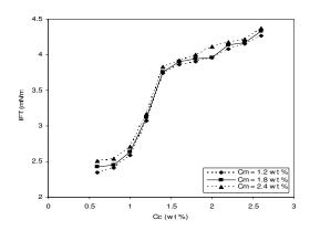
Fig. 4: IFT between brine and oil versus CaCl<sub>2</sub> concentration for three concentrations of MgCl<sub>2</sub>.
