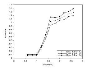
Fig. 6: IFT between polymer-contained surfactant solution and oil versus  $CaCl_2$  concentration for three concentrations of  $MgCl_2$ . Concentrations of chemicals in polymer-surfactant solution in surfactant waterfloods are: surfactant = 0.10 wt.%, xanthan = 125 ppm, and ethanol = 0.75 wt.%.
