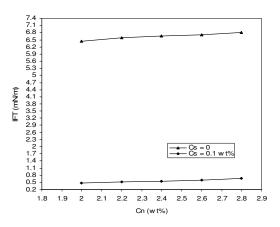
Fig. 11: Measured brine-oil and surfactant solution-oil IFT versus NaCl concentration (MgCl<sub>2</sub>: 0.5 wt.%, CaCl<sub>2</sub>: 0.5 wt.%). Concentrations of chemicals in polymer-surfactant solution in surfactant waterfloods are: surfactant = 0.10 wt.%, xanthan = 125 ppm, and ethanol = 0.75 wt.%.
