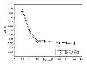
Fig. 8: Capillary number in viscous-modified surfactant waterflooding versus  $CaCl_2$  concentration  $(2^{nd}, 3^{rd}, 4^{th} \text{ ranges})$  for three concentrations of  $MgCl_2$ . Concentrations of chemicals in polymer-surfactant solution in surfactant waterfloods are: surfactant = 0.10 wt.%, xanthan = 125 ppm, and ethanol = 0.75 wt.%.
