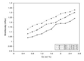
Fig. 5: Measured brine viscosity versus CaCl<sub>2</sub> concentration for three concentrations of MgCl<sub>2</sub>.
