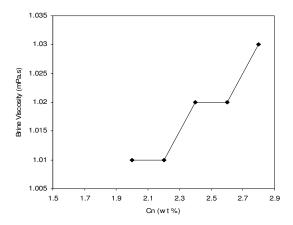
Fig. 12: Measured brine viscosity versus NaCl concentration (MgCl<sub>2</sub>: 0.5 wt.%, CaCl<sub>2</sub>: 0.5 wt.%).
