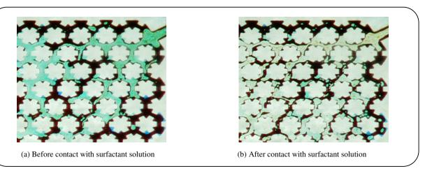
Fig. 14: Illustration of shift in wettability for micromodel (brown: oil, blue: connate water, green: waterflooding residue (brine), light grey: polymer-contained surfactant solution remained in the micromodel in the final state, white: grains). Concentrations of chemicals in polymer-surfactant solution in surfactant waterfloods are: surfactant = 0.10 wt.%, xanthan = 125 ppm, and ethanol = 0.75 wt.%.
