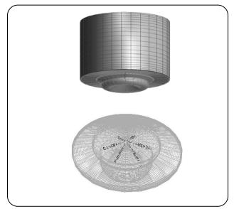
Fig. 1: Computational mesh and fuel spray at two different views.
