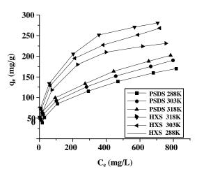
Fig. 1: Adsorption isotherms of aniline on adsorbents (Experimental conditions: absorbent 0.1g; temperature 288,303,318K; initial concentration of aniline solution 55.56, 81.50, 193.35, 406.90, 607.81, 839.95, 987.03mg/L; aniline solution100mL; time 24h.)
