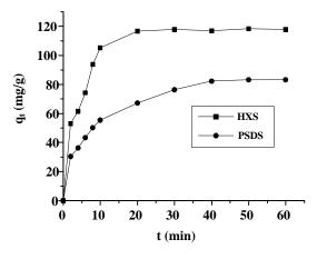
Fig. 2: Adsorption kinetics curves of aniline on adsorbents at 288K (Experimental conditions: absorbent 0.2g; initial concentration of aniline solution 193.35mg/L; aniline solution200mL; temperature 288K).
