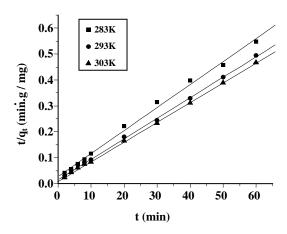
Fig. 3: Adsorption kinetics fitted curves of aniline on HXS fiber (Experimental conditions: absorbent 0.2g; initial concentration of aniline solution 193.35mg/L; aniline solution200mL; temperature 283,293,303K).
