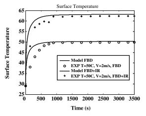
Fig. 5: Comparison between experimental and predicted surface temperature of green peas sample in both systems, FBD & FBD+IR (T=50 °C, V=2m/s, Mip =400g, dia=9mm).
