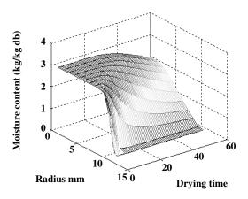
Fig. 6: Development of the moisture distribution in green peas sample during drying in fluidized bed dryer assisted by infrared heat source (T=50 °C,  $M_{ip}=400g$ , dia=10mm, Power=600W, V=3m/s).
