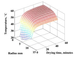
Fig. 7: Development of the temperature in green peas sample during drying in fluidized bed dryer assisted by infrared heat source (T=50 °C,  $M_{iv}=400$ g, dia=10mm, Power=600W, V=3m/s).
