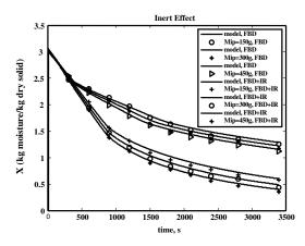
Fig. 11: Experimental and predicted average moisture contents of green peas in three different amounts of inert particle 150, 300 and 400 g in both systems (FBD & FBD+IR).
