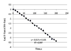
Fig. 3: Plot of Ln(dimensionless temperature) vs time for determination of total heat transfer coefficient in a 2 cm diameter of aluminum sphere.
