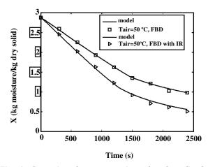
Fig. 4: Comparison between experimental and predicted average moisture contents of green peas sample in both system FBD & FBD+IR (T=50 °C, V=2m/s, Mip =400g, dia=9mm).
