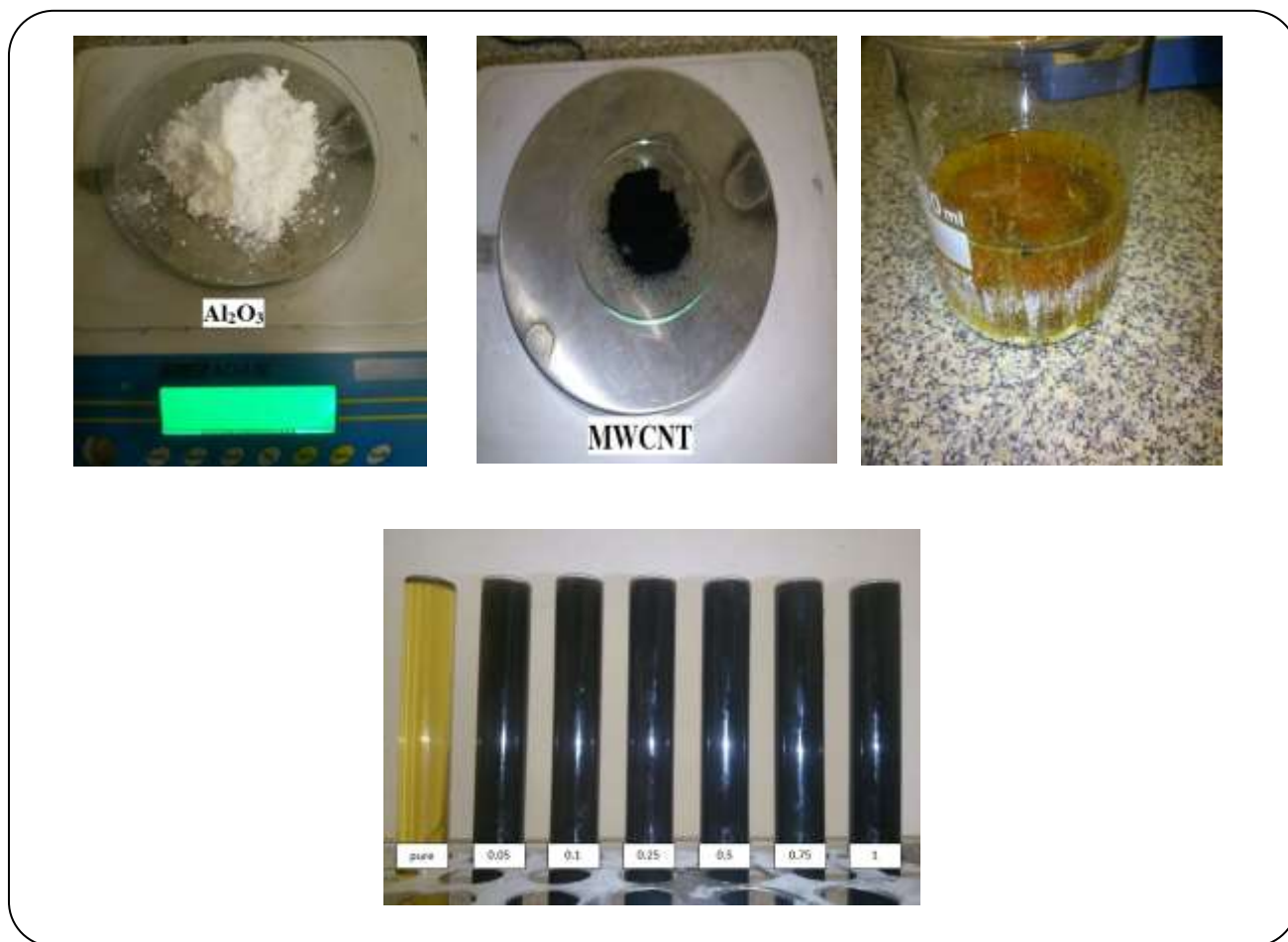
Fig. 1: Photograph of Al_2O_3 and MWCNT particles, 10W40 and nano-lubricant samples.
