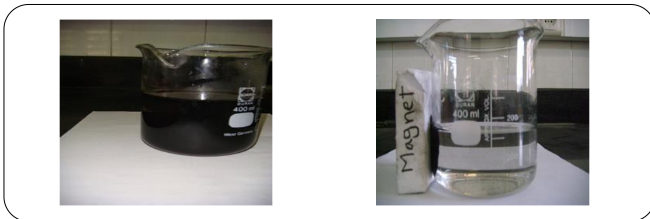
Fig. 8: Separation of Fe_3O_4@SiO_2@meso-SiO_2 from water by a magnetic field
