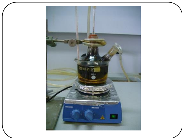
Fig. 1: Experimental set-up for the preparation of magnetic core-mesoporous shell.
