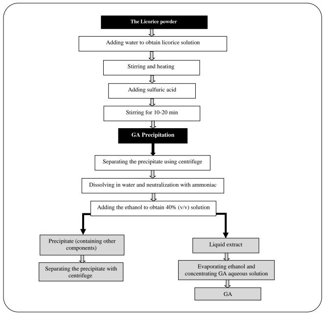
Fig. 1: The diagram of Glycyrrhizic acid extraction procedure.
