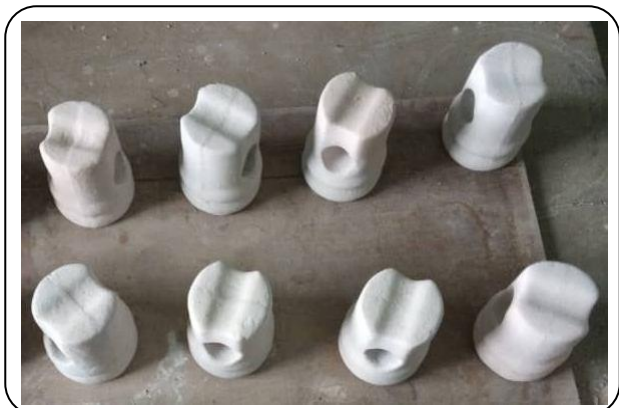
Plate 1 low voltage pin porcelain insulators bisque fired at 900°C
