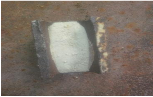
Plate 1 Test result of sample A (silica without flux) fired at 1200°C
