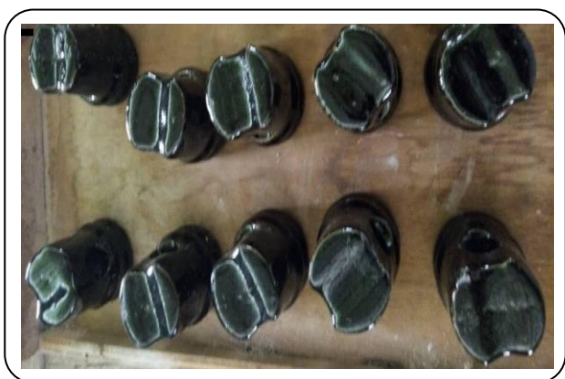
Plate 2 Low voltage pin porcelain insulators fired gloss at 1200° C
