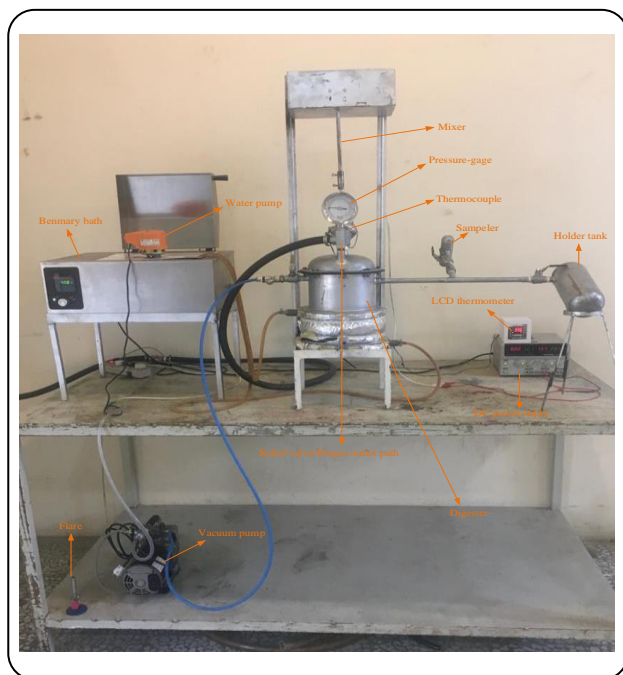
Fig. 1: Anaerobic digestion equipment set.
