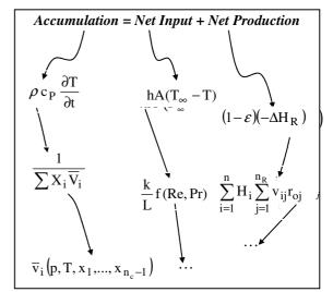
Fig. 5: Energy balance equation for a reactor and a possible decomposition of its quantities
