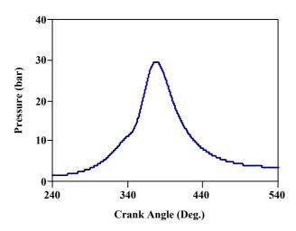
Fig. 4: Cylinder pressure variation (Simulated).
