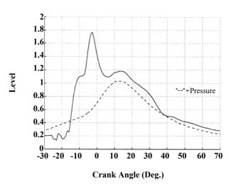
Fig. 10: Normalized ion current and pressure variation via crank angle (Experimental).
