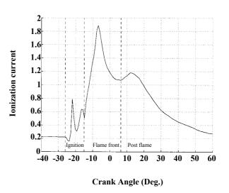
Fig. 2: Ionization current signal characteristic in three phases: Ignition, Flame front and Post flame.
