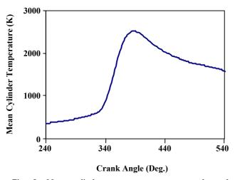
Fig. 5: Mean cylinder temperature verses crank angle (Simulated).
