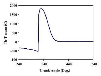
Fig. 7: Burned gas and cylinder mean temperature difference variation verses crank angle (Simulated).
