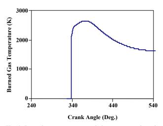
Fig. 6: Burned gas temperature variation verses crank angle (Simulated).
