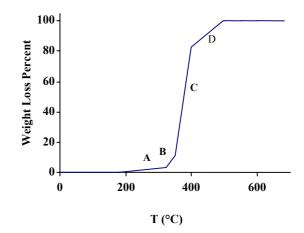
Fig. 4: The TGA graph of synthesized silicalite-1.
