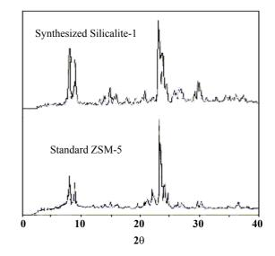
Fig. 5: XRD patterns of synthesized silicalite-1 and standard ZSM-5.
