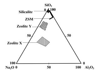
Fig. 2: Ternary composition diagram of  $Na_2O-Al_2O_3$ -SiO<sub>2</sub> system for synthesis of silicalite.
