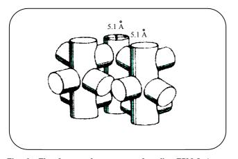
Fig. 1: The framework structure of zeolite ZSM-5 ( or Silicalite ).
