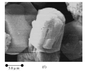
Fig. 6: The scanning electron micrographs of : (a) cyclic alpha quartz, (b) ovate alpha quartz, (c) prolonged ovate alpha quartz, (d) and (e) coffin shape silicalite-1 (SiO<sub>2</sub>:Na<sub>2</sub>O molar ratio 50:2.04), (f) coffin shape silicalite-1 (SiO<sub>2</sub>:Na<sub>2</sub>O molar ratio 50:4.10).
