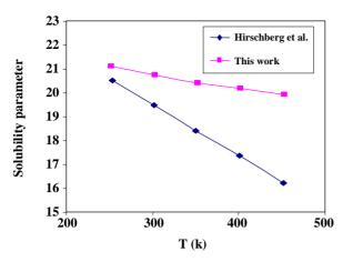
Fig. 5: The effect of temperature on the asphaltene solubility parameter calculated by the modified PR EOS and by Hirschberg et al.'s correlation.
