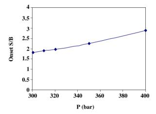
Fig. 4: The effect of pressure on the onset solvent-to-bitumen ration.
