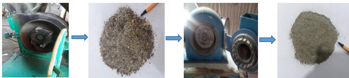
Fig. 1: Primary and secondary crushing of the representative sample and dimensions of the crushed sample.
