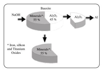
Fig. 1: Aluminium oxide is dissolved out of the bauxite and processed further to aluminium. The residue containing a mixture of naturally occurring minerals is then transferred to a disposal site.
