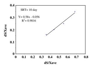
Fig. 3: Determination of Y and  $k_d$  in SRT =10 days. Under noozone-addition condition.
