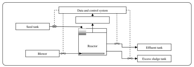
Fig.1: The general view of SBR schematic.
