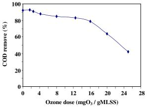
Fig. 4: The effect of ozone does on COD removal efficiency.
