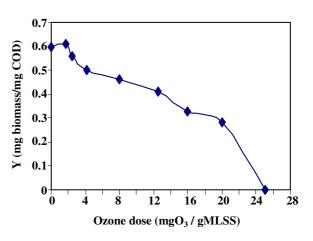
Fig. 7: The effect of Ozone does on Y.
