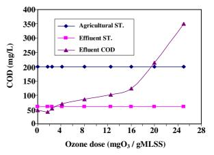
Fig. 8: Compare of Effluent Wastewater COD removal by different ozone dosage with Iran wastewater reuse standard for agricultural reuse.
