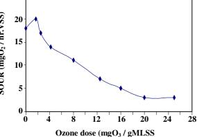
Fig. 6: The effect of Ozone does on SOUR.
