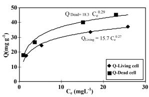
Fig 3:  $Ni^{2+}$  adsorption isotherms of 0.1 mol  $L^{-1}$  HCl-treated cell and living cell in the rapid phase.
