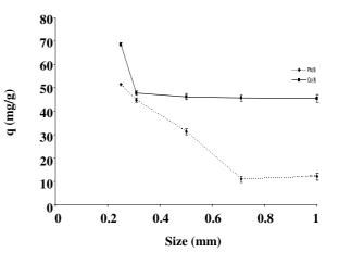
Fig. 2: Effect of biosorbent size on uptake of Pb(II) and Co(II) by RRWB
