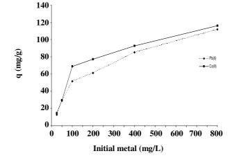
Fig. 3: Effect of initial metal concentration for uptake of Pb(II) and Co(II) by RRWB.
