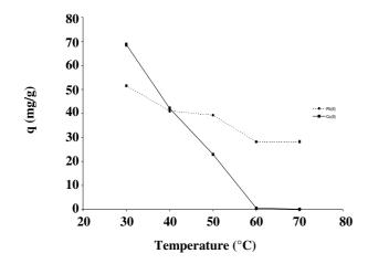
Fig.4: Effect of temperature for uptake of Pb(II) and Co(II) by RRWB.
